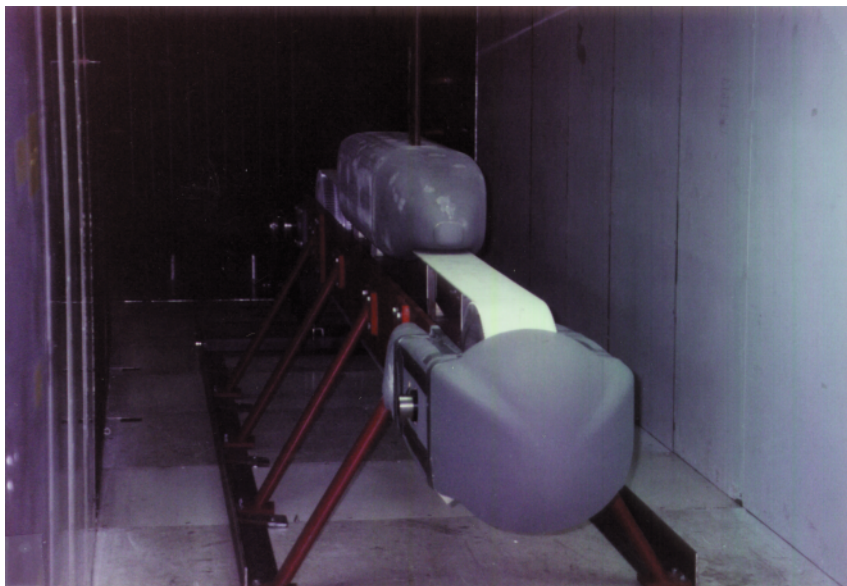
Figure 22 The elevated moving track Maglev test apparatus in the Virginia Tech 6 ft \times 6 ft wind tunnel with an electromagnetic suspension (EMS) system model mounted over the belt.
