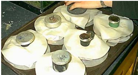
Figure 3. Saturating specimens wrapped in filter paper.
