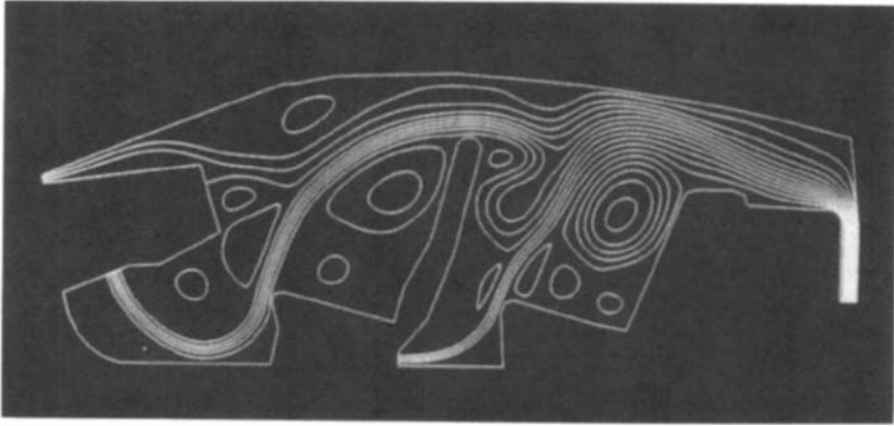
Figure 30 Streamlines inside a passenger compartment without passengers; laminar flow.
