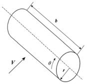
To calculate  $C_D$  using the data obtained in the lab, plot  $C_p \cos\theta$  vs.  $\theta$  and integrate the area under the curve. Use any numerical or graphical integration technique.
