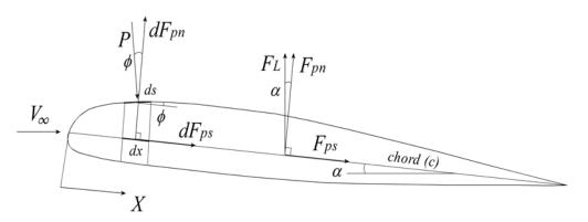
The total pressure force normal to the chord is the difference between the corresponding pressure forces acting on the lower and upper surfaces,
