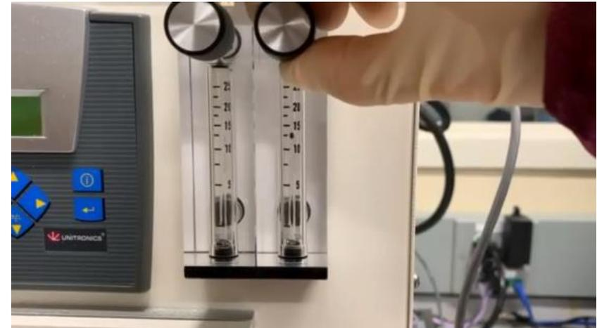
Note: Adjust gas flow until desired chamber pressure is achieved (you can check pressure of chamber by pressing 'left arrow')
