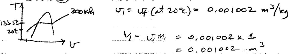
At ②, P<sub>2</sub> > P<sub>Lift</sub>  $\Rightarrow$  PISTON IS AGAINST STOPS
