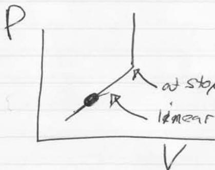
for a spring loaded piston/cyl.
