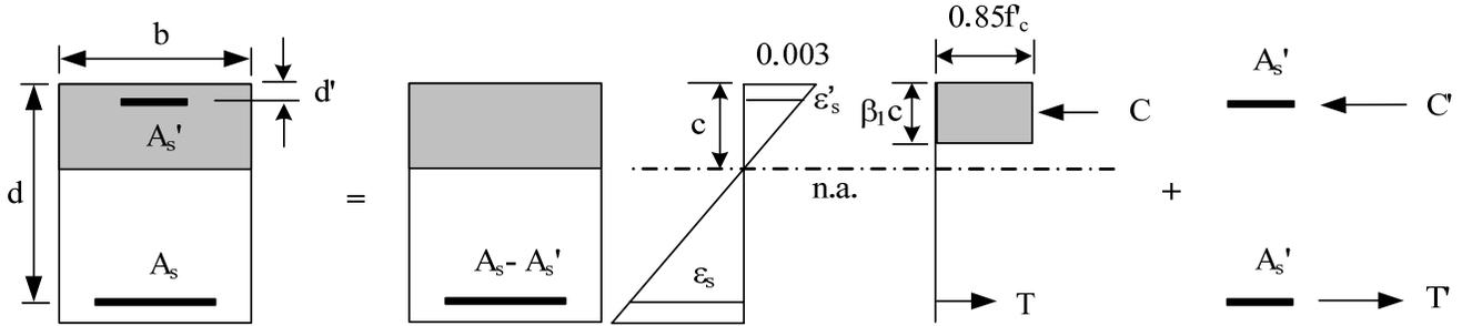
Fig. 1-3 A rectangular section with compression reinforcement
