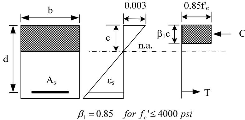
Fig. 1-1 Ultimate strain profile and corresponding rectangular stress distribution
