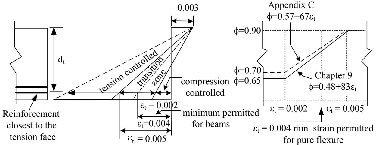
Fig. 1-2 Capacity reduction ( $\phi$ ) factors for Grade 60 reinforcement
