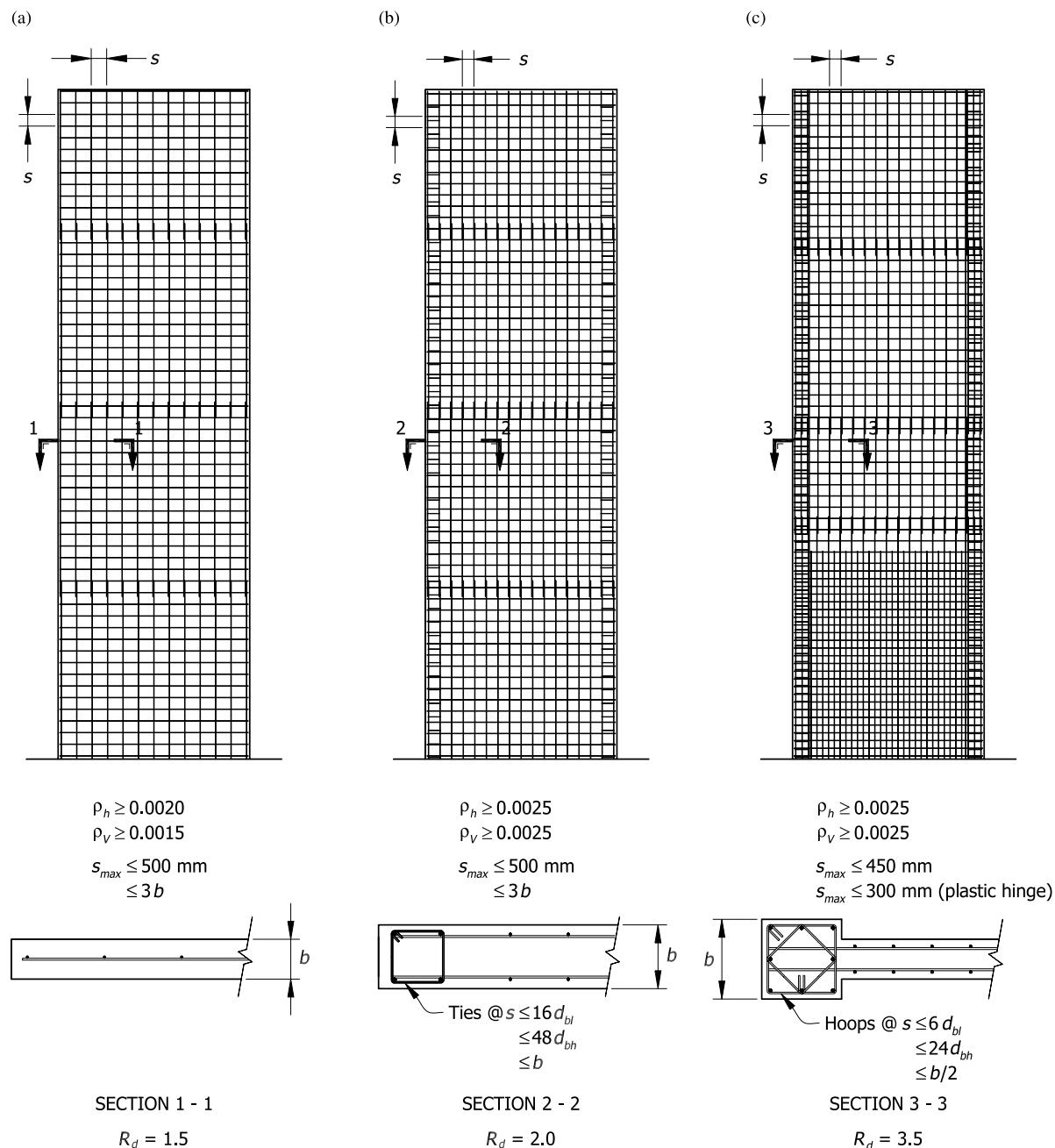
level. Walls with moderate ductility ( $R_d = 2.0$ ) must be capable of developing some flexural hinging at the base of the walls without significant shear distress, must satisfy minimum ductility requirements, and must satisfy minimum detailing requirements specified in clause 21 of CSA-A23.3-94.
