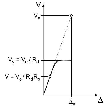
or minimum overstrength may be used. For a particular structural system, this dependable overstrength arises from the application of the design and detailing provisions prescribed in the appropriate CSA standard. The proposed 2005 NBCC has overstrength factors,  $R_o$ , that have been determined in a consistent manner for all systems in conformance with the CSA provisions.
