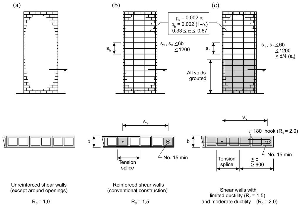
**Fig. 13.** Summary of detailing requirements for masonry moment-resisting frames (CSA 1994b).  $d_{bt}$ , diameter of lateral ties.
