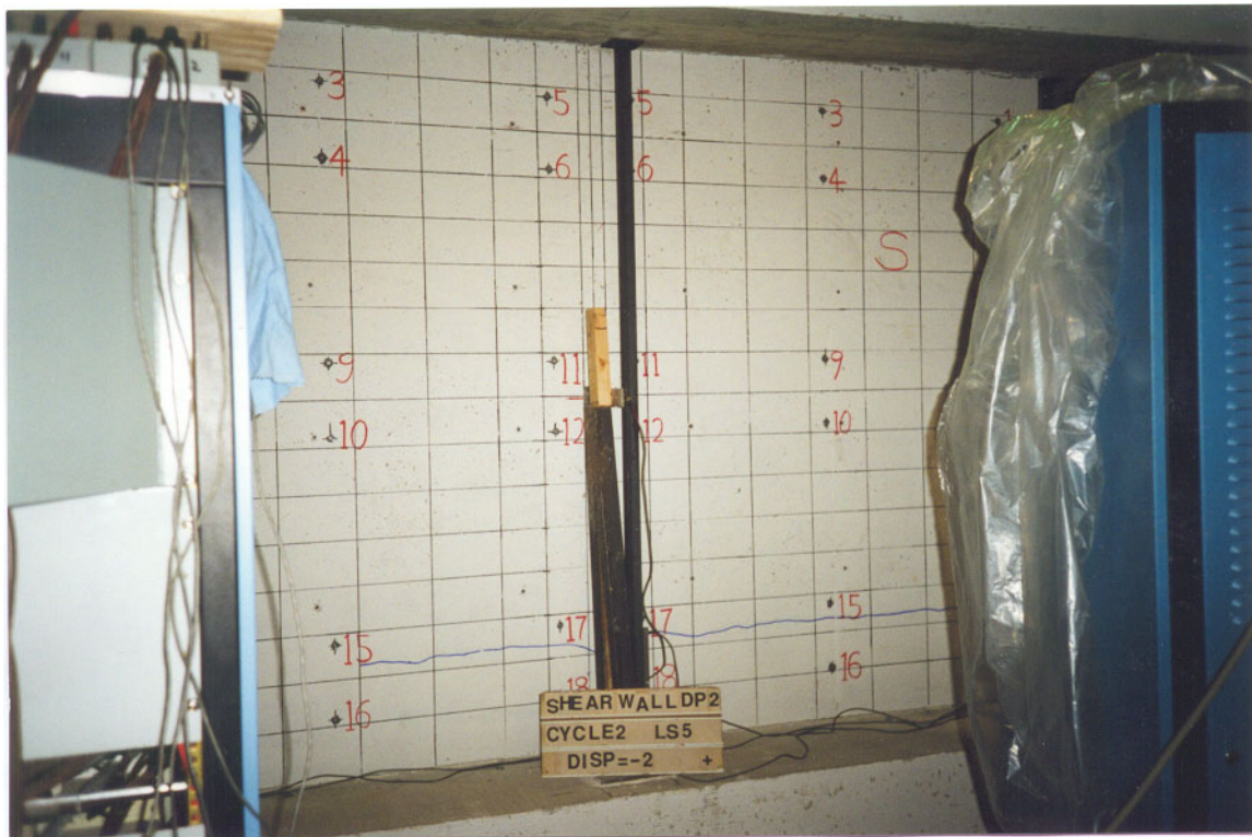
Figure 5.11 DP2 Flange Wall After 2 mm Lateral Displacement
