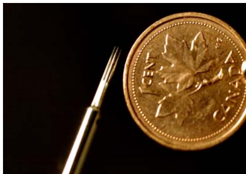
Four-sensor cold-wire probe: 0.7 \mu\text{m} dia, 0.5 mm length
