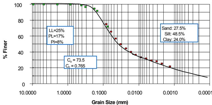
FIGURE 3. Grain size analysis for Botkin soil.
