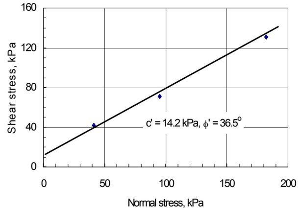
FIGURE 9. Direct shear test results to determine the saturated shear strength parameters of the Botkin silt
