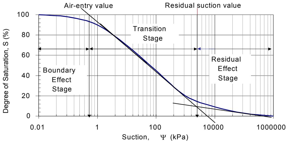
FIGURE 1. Typical soil-water characteristic curve showing various stages.
