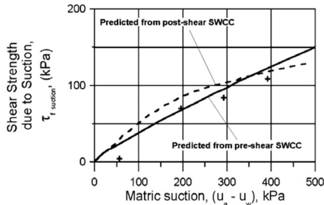
Figure 6. Measured and predicted shear strength of Dhanauri clay for a suction range of 0 to 400 kPa and a net confining pressure of 386kPa
