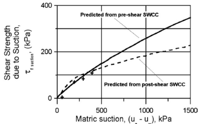
Figure 7. Measured and predicted shear strength of Dhanauri clay for a net confining pressure of 386kPa
