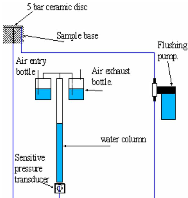
Figure 9. Detail of the flushing system.
