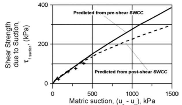
Figure 4. Measured and predicted shear strength of Dhanauri clay for a net confining pressure of 96 kPa.
