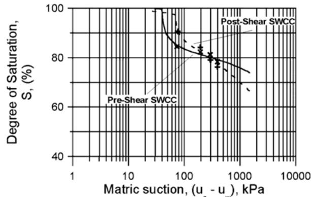
Figure 2. Soil-water characteristic curve data derived from the triaxial shear test results undertaken on Dhanauri clay specimens tested under a confining pressure of 96 kPa.
