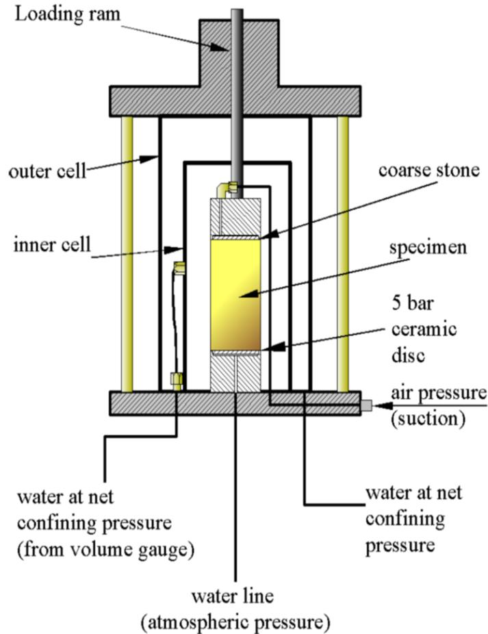
Figure 8. Modified triaxial cell for determining the shear strength of unsaturated soil specimens.
