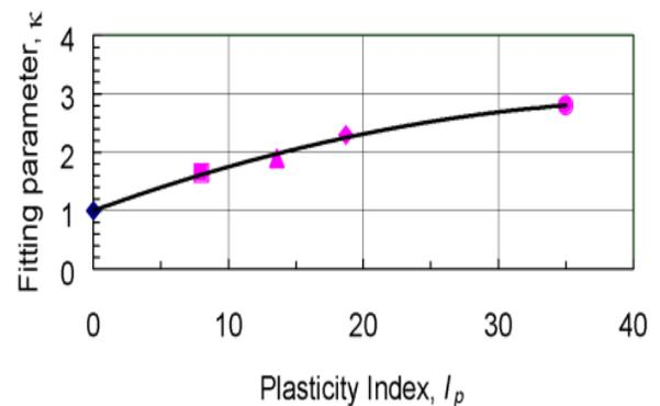
Figure 1. Relationship between the fitting parameter  $\kappa$  and the plasticity index of a soil (from Vanapalli and Fredlund, 2000)
