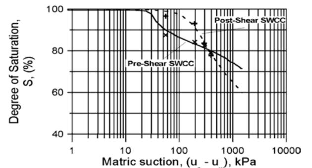
Figure 5. Soil-water characteristic curve data derived from the triaxial shear test results undertaken on Dhanauri clay specimens tested under a net confining pressure of 386 kPa.
