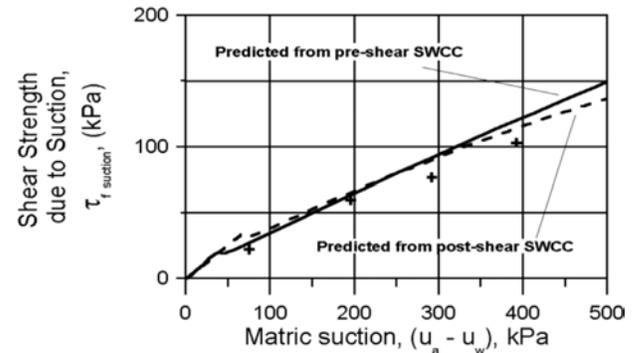
Figure 3. Measured and predicted shear strength of Dhanauri clay for a suction range of 0 to 400 kPa and a net confining pressure of 96kPa.
